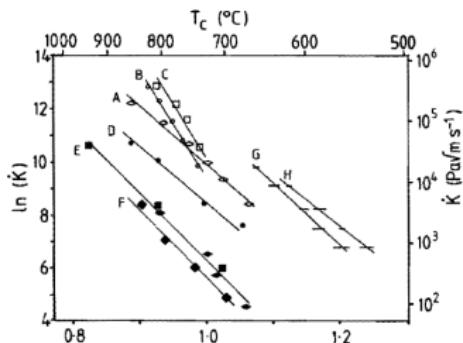
Brittle to ductile transition temperature of silicon
